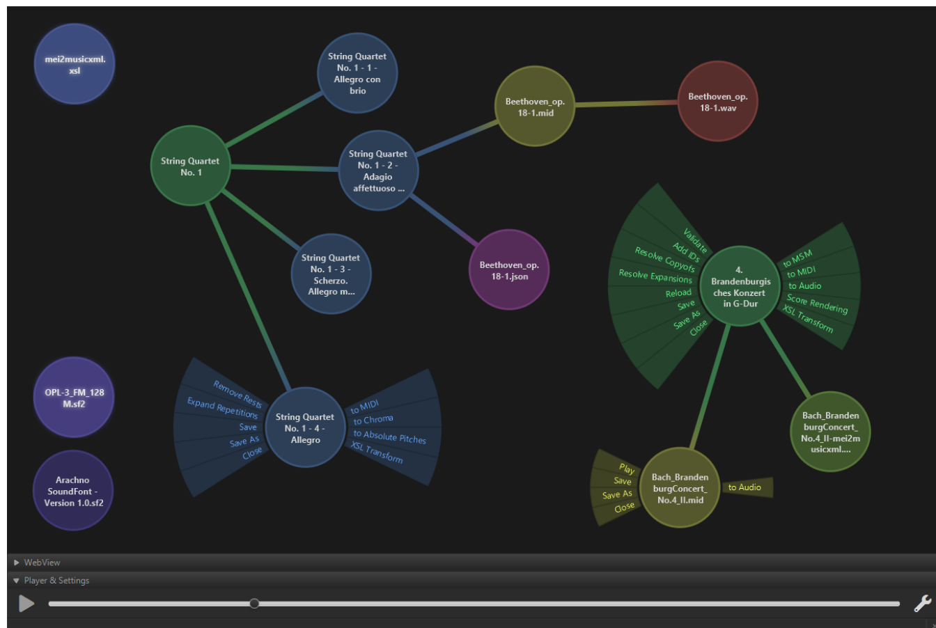
Figure 2: After several extensions of meico’s functionality conversion paths became more branched deeming the first revision graphical user interface inappropriate. The second revision GUI, shown here, presents a graph visualization of conversion paths, more accessible functionality via radial menus, a more advanced audio and MIDI player, and an integrated WebView to access online services such as the Verovio score rendering.
